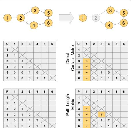
**Fig. 1.** Computing BA and OBA. Without node 2, five paths would be longer (hence less efficient) or impossible (1>3..6; 3>4). This can be implied by the two path length matrices on the bottom. BA accumulates to 5. Four of those connections would not be connected at all (1>3..6). Thus OBA = 4
