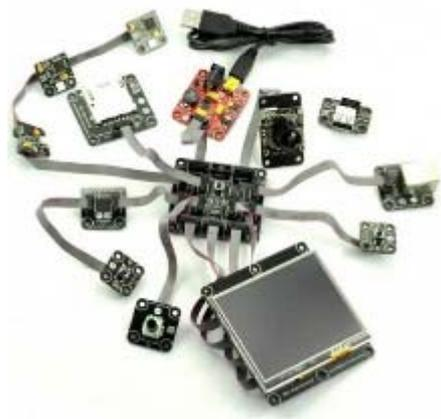
**Fig. 2:** FEZ Spider Kit by GHI Electronics. An example of modular .NET Gadgeteer hardware.
