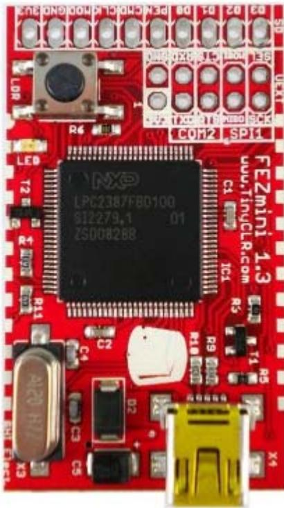
**Fig. 1:** FEZ Mini by GHI Electronics. One of the smallest development boards with an LPC2387 system on chip. 72 MHz, 96 kB RAM, 512 kB FLASH.
