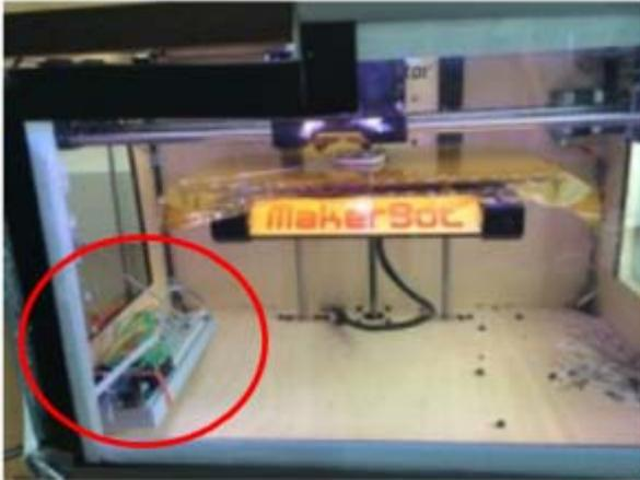
**Figure 2:** Integrated Arduino Board with different sensor capabilities
