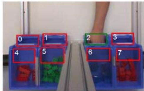
**Figure 2:** A graphical user interface is used to define interactive zones. (Here in an assembly context)
