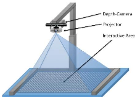
**Figure 1:** Our prototypical setup uses a depth camera to survey zones and a projector to display feedbacks
