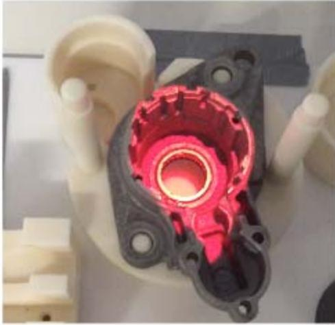
**Figure 3:** An object needs to be placed at a storing area. The shape and the position of the projected red light indicates the position and orientation of the object.
