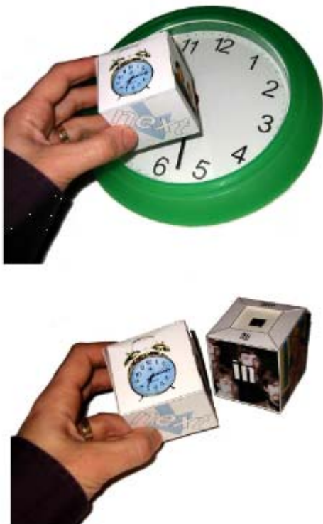
Figure 1: Use of the deictic references in the tangible IoT programming language Media Cubes , designed for end-user scripting in AutoHAN [4].
