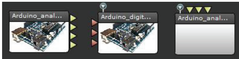
Figure 3: From left to right: (1) node for retrieving analog sensor input from the Arduino Duemilanove board, (2) node for writing digital values, (3) experimental node for writing analog values
