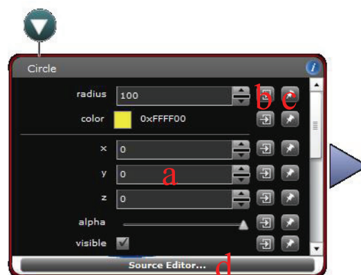
Figure 2: Attribute inspector of one node (second state of a node). (a) Attributes can be modified directly, (b) be bound to the output of another node or (c) be published to the global attributes panel for direct modification within the whole composition. (d) The source editor (third state of a node) is accessible at the bottom of the node.
