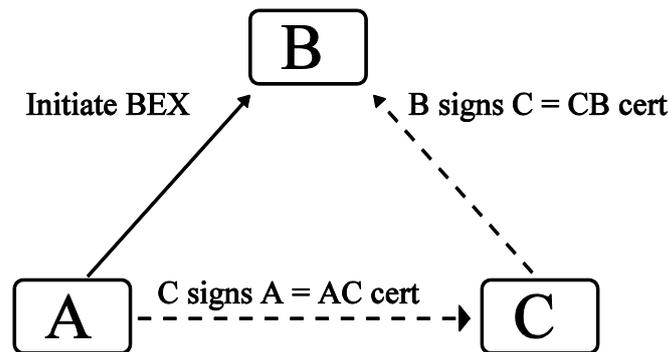
Figure 1 Forming of a trust relationship between host A and host B by presenting the certificate given to host C to host A.
