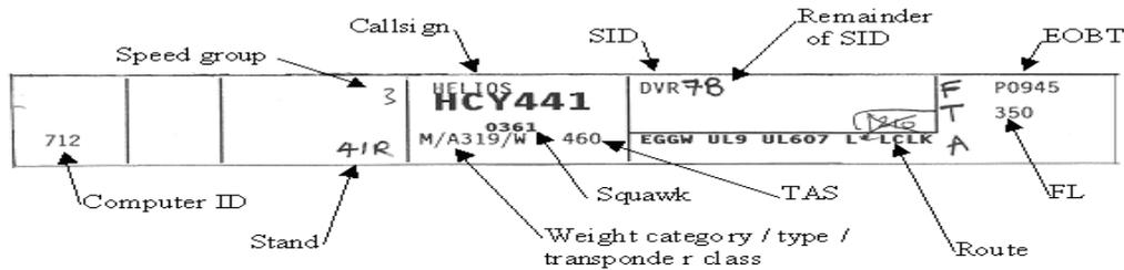
Figure 3. Flight Progress Strip
